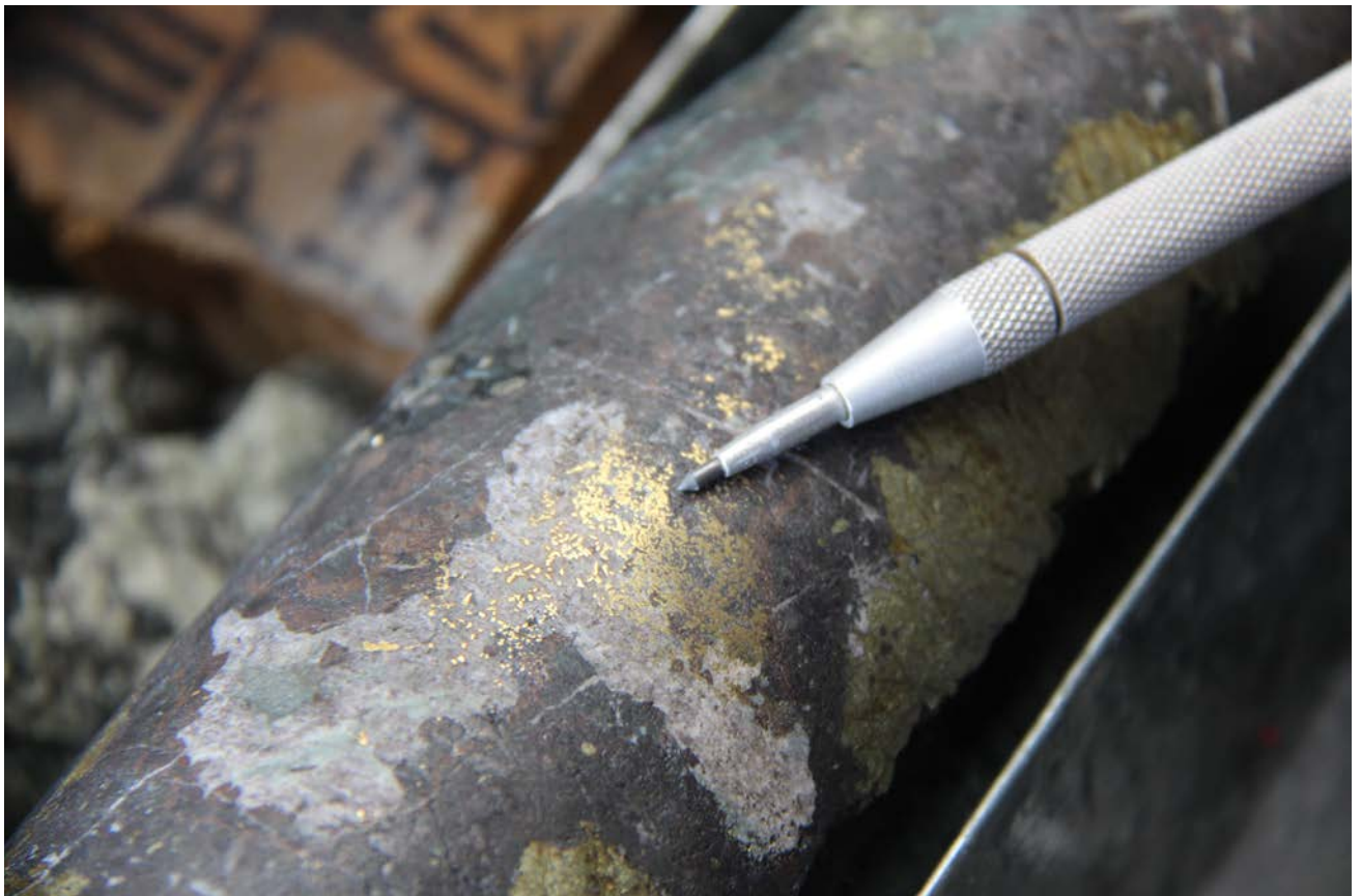
Figure 1: Image of strong coarse visible gold in sphalerite-carbonate vein cutting chalcopyrite in ACD036
