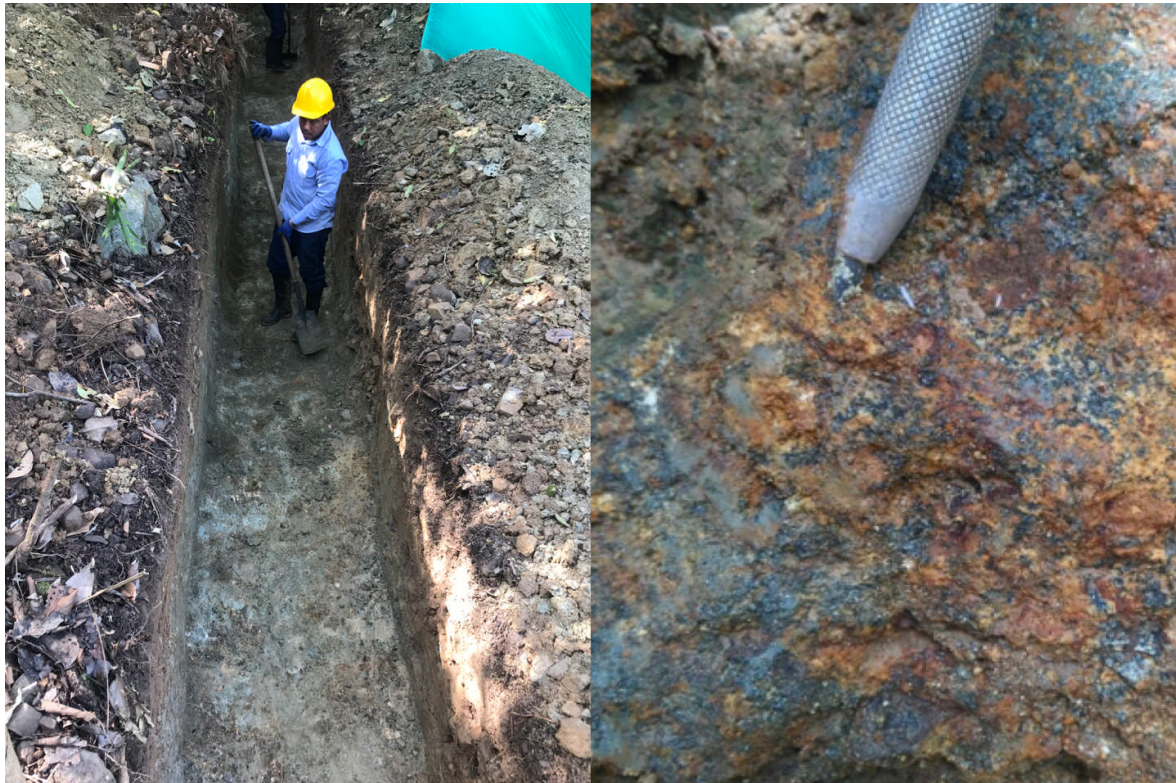
Figure 3: Trenching activity in the Buenos Aires area (left) and massive sulphides discovered at the Buenos Aires South structure (right).
