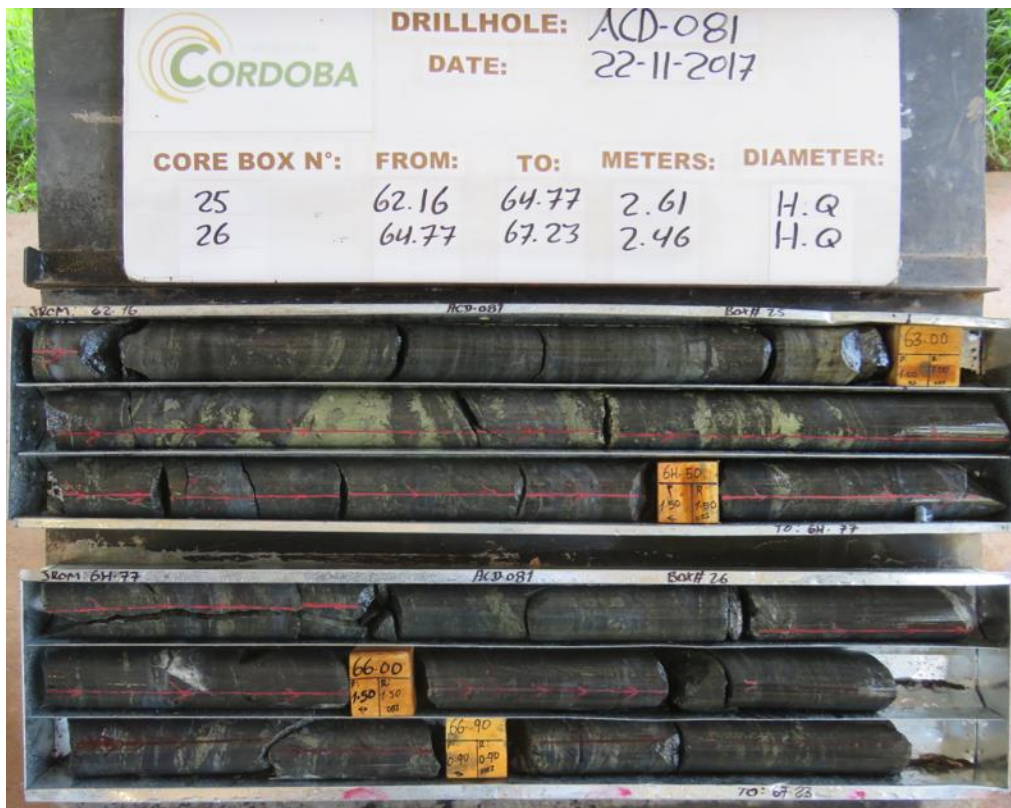
Figure 5: Example of high-grade mineralization in hole ACD081 with 5.99% copper and 1.99 g/t gold over 1.0 metres ( 7.50% CuEq ; from 63m)
