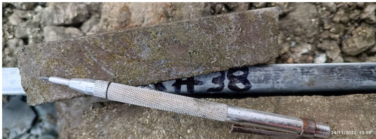
Figure 4: Hole ACD147 at 105.5 m showing fine tuff replaced with semi-massive pyrite, chalcopyrite and pyrrhotite. This sample was part of a 1 m interval from 105.50 m to 106.50 m, which returned 1.93% Cu, 0.88 g/t Au, 11.45 g/t Ag, or 2.39% CuEq 1 .
