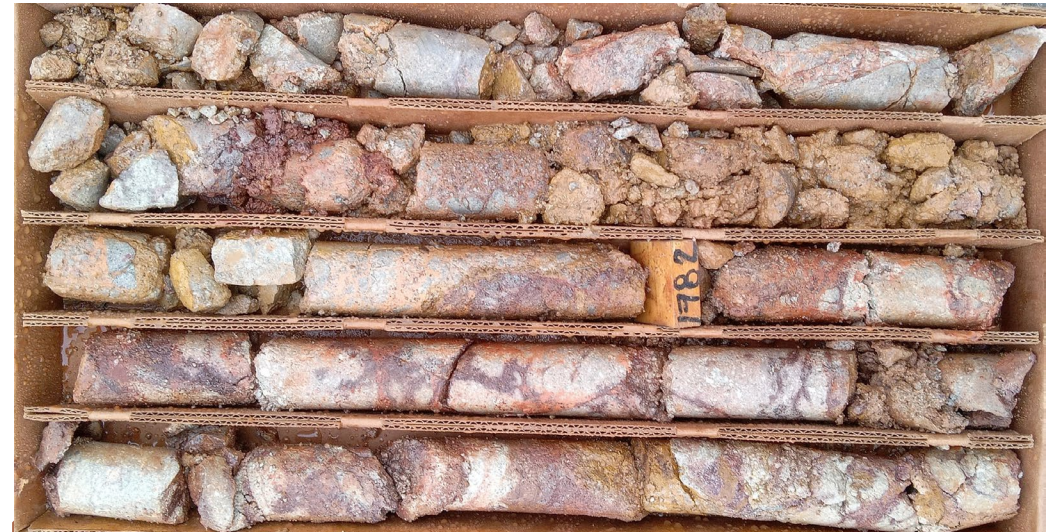
K-23 at 543 meters showing hematitic leached capping hosted in strongly sericitized Laramide volcanic tuff
