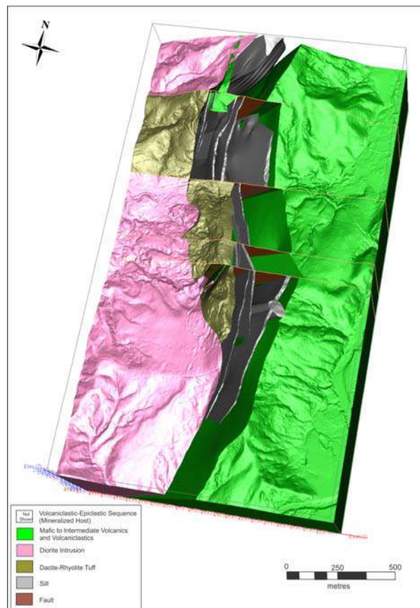
Figure 1: Plan view of Alacran geological model showing generally west-dipping lithostratigraphy, with mafic to intermediate volcanics & volcanoclastics in the east and footwall to the main copper-gold mineralised zones hosted mainly by avolcaniclastic -epiclastic sequence that is intruded by intermediate sills and also larger dioritic bodies in the west and north. Mineralization also locally overprints the intrusions.
