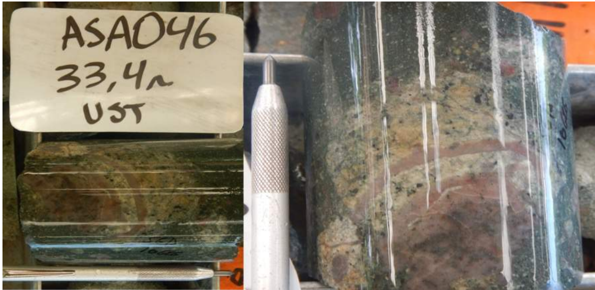
Figure 9: Unidirectional Solidification Textures.
