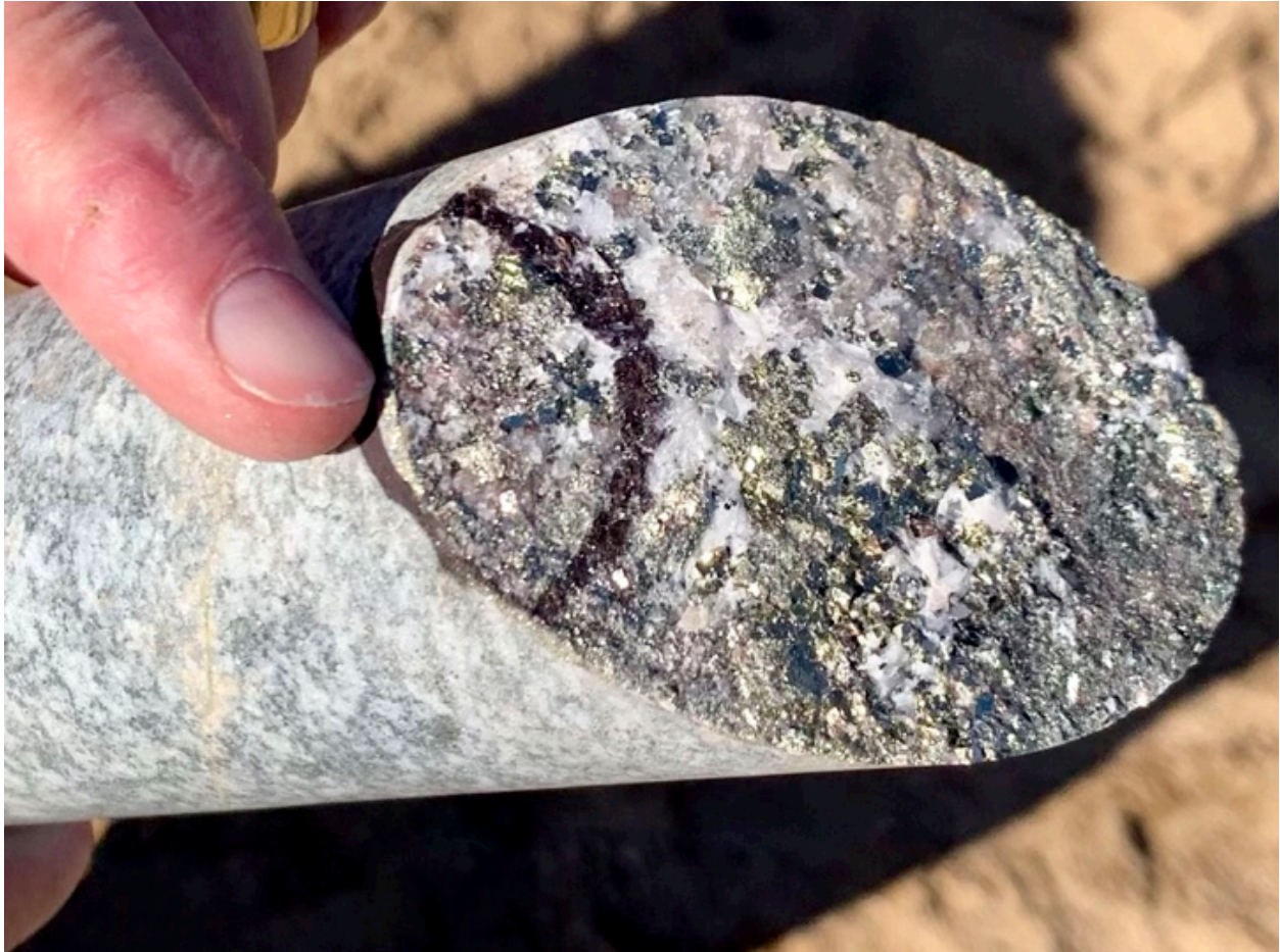
Figure 3* : Bornite and chalcopyrite mineralization along fracture plane at approximately 1,020 metres.
