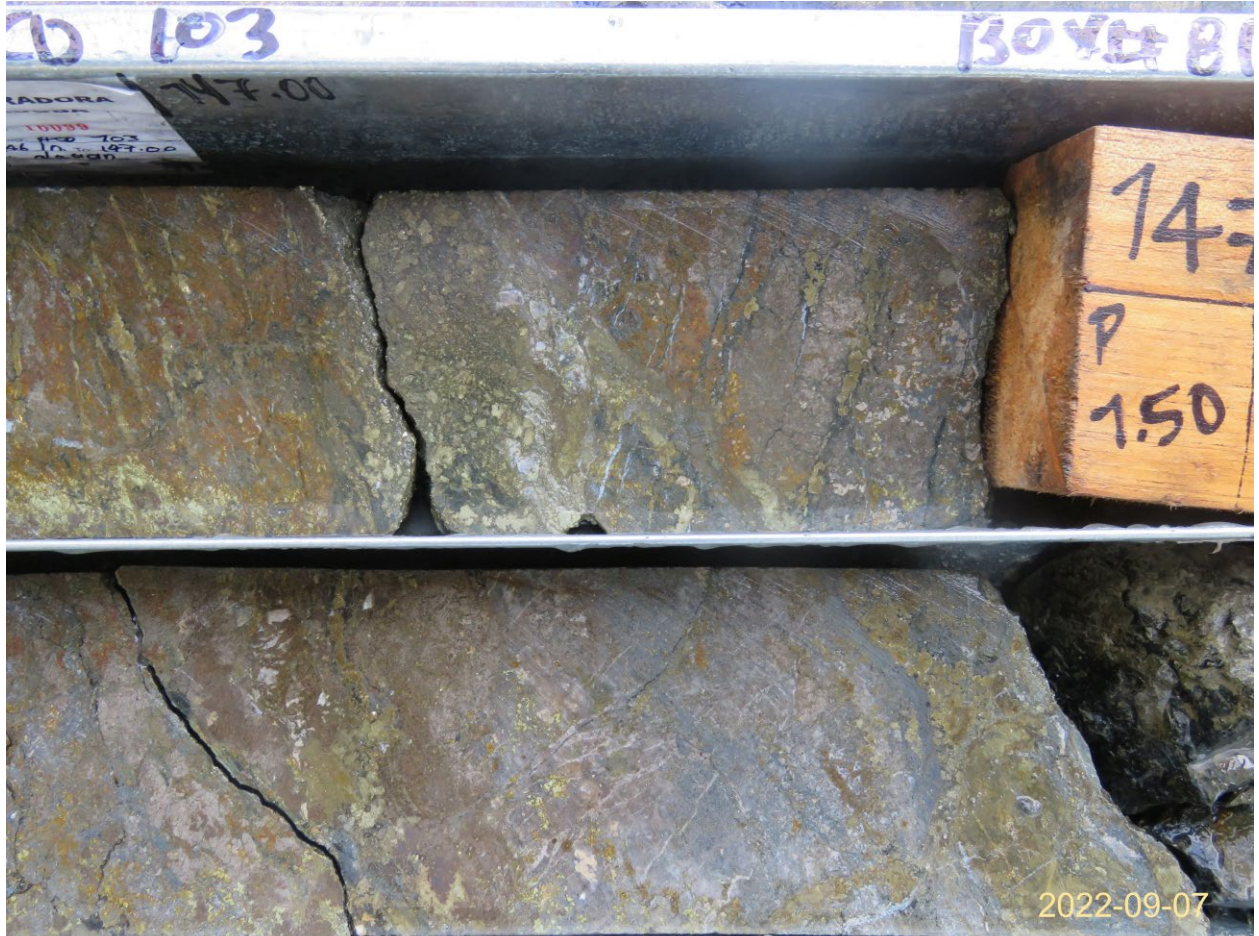
Figure 10: Semi-massive chalcopyrite and pyrite within 'Unit 2' carbonaceous mudstones at 147 m below collar in hole ACD103. This sample returned 7.98% Cu, 1.995 g/t Au and 42.6 g/t Ag for 8.85% CuEq 1 and is at the base of a 33.78 m higher grade zone between 114.12 m and 147.90 m below collar which returned 1.31% Cu, 0.41 g/t Au and 6.77g/t Ag or 1.50% CuEq 1 .
