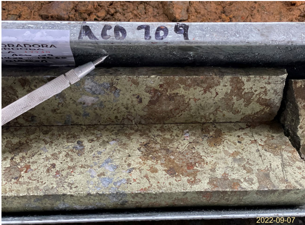
Figure 11: An example of high grade CBM vein mineralization with massive chalcopyrite, pyrite, pyrrhotite with minor magnetite at 136 m below collar in ACD109. This sample returned 11.85% Cu, 5.47 g/t Au and 144 g/t Ag for 15.16% CuEq 1 within a 30.48 m higher grade zone between 115.90 m and 146.38 m below the collar; assaying 1.87% Cu, 1.00 g/t Au, 16.69 g/t Ag or 2.43% CuEq 1 .
