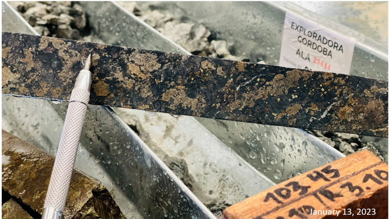
Figure 4: Hole ACD157 at 103.45 m showing a volcanic tuff within 'Unit 2', with a very fine dark coloured matrix of ash and lapilli, some carbonate fragments, and semi-massive sulfides, such as pyrite and chalcopyrite replacing the matrix. This sample was part of a 44 m interval from 84.30 m to 128.30 m, which returned 1.79% Cu, 0.62 g/t Au, 11.96 g/t Ag, or 2.11% CuEq 1 .
