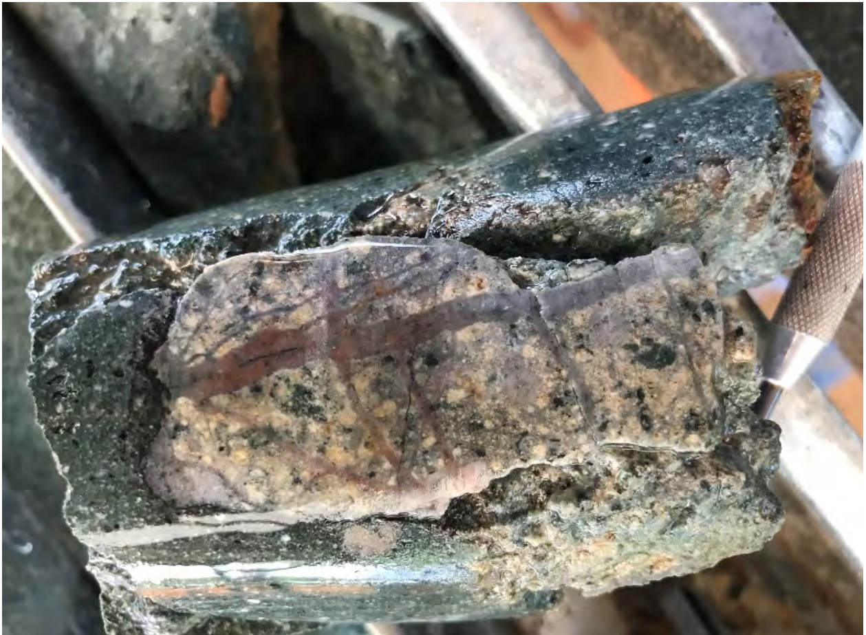
Figure 9-17: IOCG/CRD clast with A-type veins in dacite breccia in Alacran deposit drill core hole ASA-046
